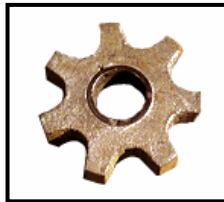
Figure 1 An idler with corrosive wear
