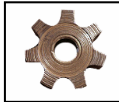
Figure 2 An idler with wear from large abrasive particulate
